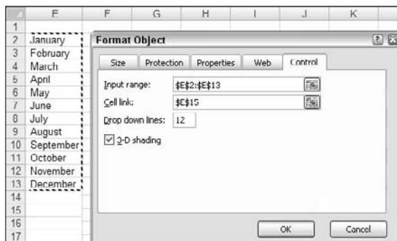
Figure 11-16: Formatting the Combo Box control.
