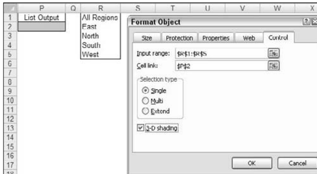
Figure 11-27: Add a List Box and note the cell where the output value will be placed.
