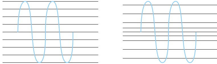
FIGURE 11.25 a. Pulse Amplitude Modulation b. Pulse Code Modulation
