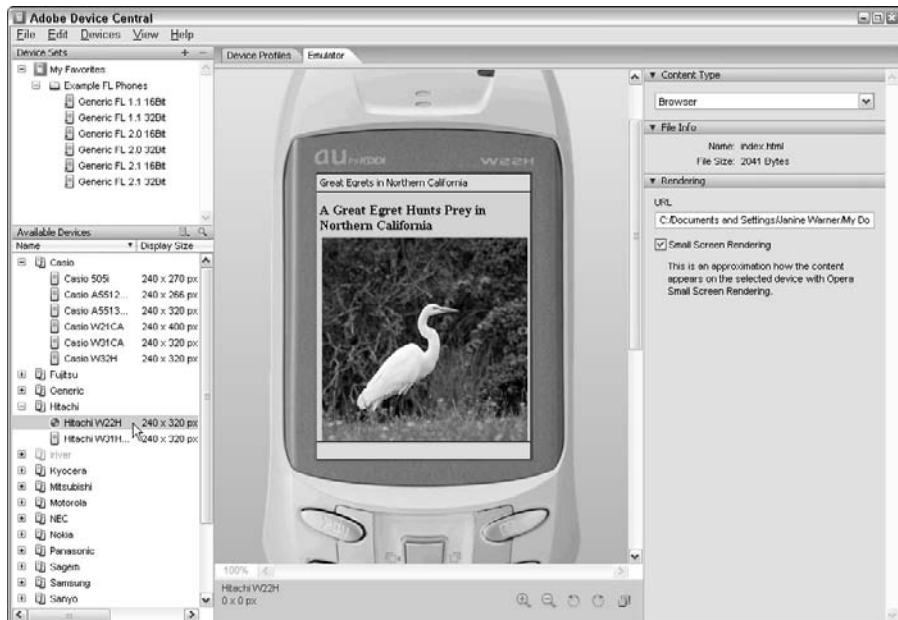
Figure 2-15: Adobe Device Central is a new emulator included in Dreamweaver CS3 to make it easy to test your Web pages in a variety of cell phones and other devices.
