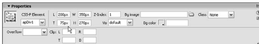
Figure 6-19: Change the height and width of an AP Div in the Property inspector.
