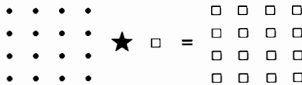
b. Convolution of an object with a periodic array of delta functions.
