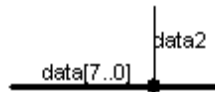
Figure A.7 A single connection line connected to an 8-bit bus with the name data .
