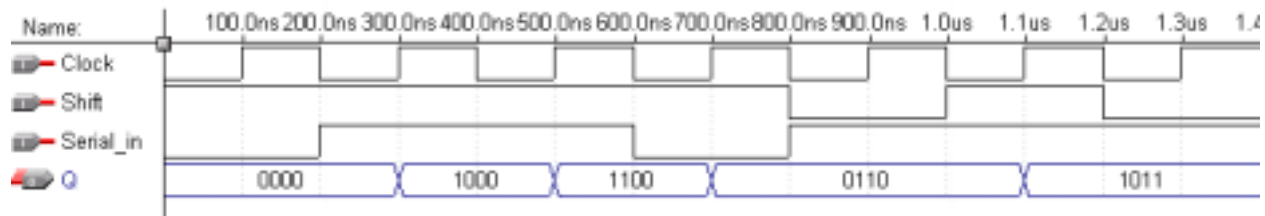
Figure 8.6 Sample simulation trace for the 4-bit serial-in-parallel-out shift register of Figure 8.5.
