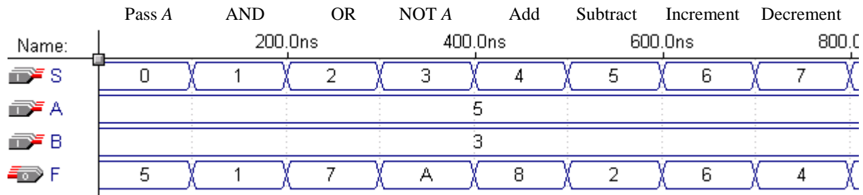
Figure 4.14 Sample simulation trace with the two input operands 5 and 3 for all of the eight operations.
