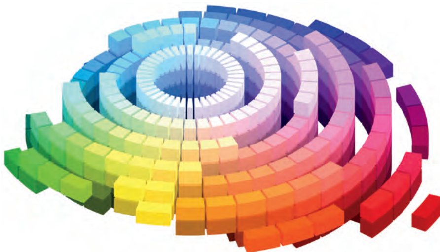
FIGURE 8-14 Because of the perceptual uniformity of the Munsell system, some colors have wider ranges of value and chroma. The color space itself is not uniform in shape. SharkD ( http://commons.wikimedia.org/wiki/User:SharkD )
