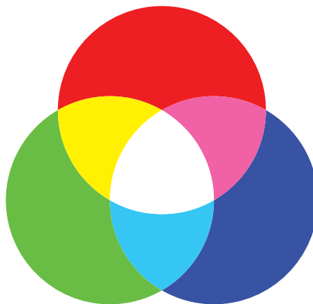
FIGURE 8-26 In an additive color model, red, green, and blue light mix together to make white.
