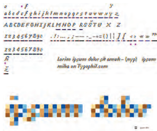
FIGURE 3-24 Subpixel typefaces exploit the red, green, and blue stripes within the pixels on LCD screens to render tiny type.
