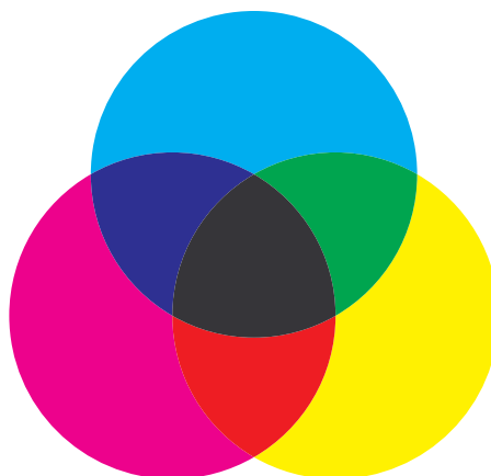
FIGURE 8-36 How cyan, magenta, and yellow ink – part of the subtractive CMYK color model – mix.
