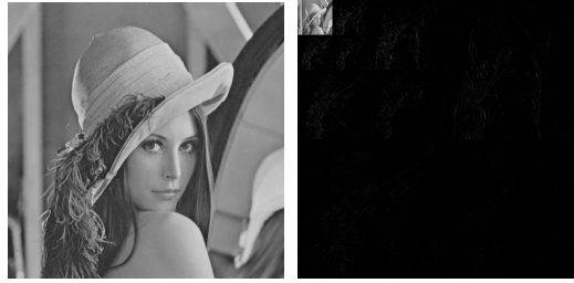
Fig. 2 Example of DWT result (Left: original Lena image. Right: 3-level DWT result)
