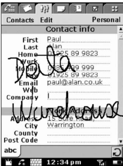
FIGURE 26.40 Write-anywhere text input method for mobile devices. Example of an Address Book application with the Company field appearing with focus. Handwritten input is not restricted to a delimited area of the screen but rather can occur anywhere. The company name Data Warehouse has been written.
