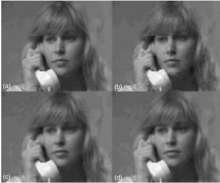
FIGURE 26.29 150th Frame of original: (a) “Suzie” sequence and its compressed version at 64 kbit/s using, (b) H.261, (c) baseline H.263, and (d) Full-option H.263.
