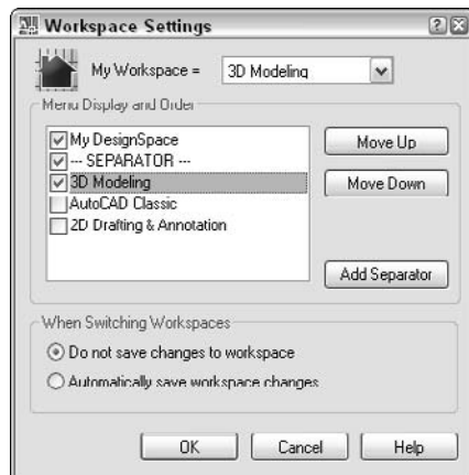
Figure 3-6: The Workspace Settings dialog box allows you to organ- ize your workspaces.
