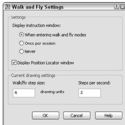
Figure 5-8: Adjust the settings for the Walk and Fly commands by using the Walk and Fly Settings dialog box.
