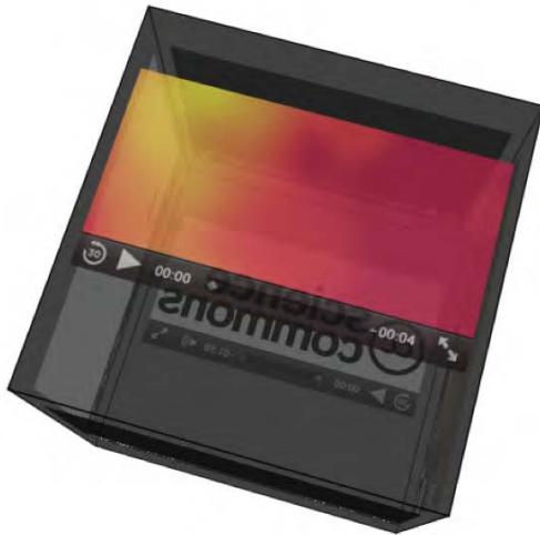
Figure 3–16. A spinning video cube fully created in CSS with animations in Safari
