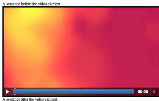
Figure 3–4. A <video> in Chrome with display set to block in surrounding inline text
