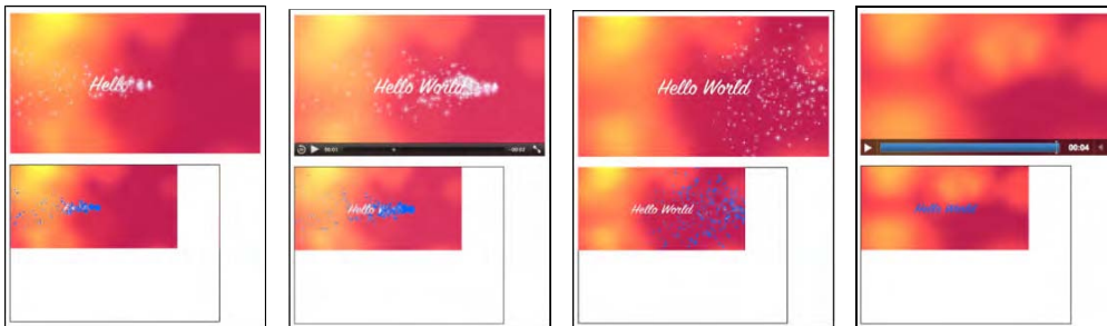
Figure 7-3. Motion detection results on a video using Web Workers in Firefox, Safari, Opera, and Chrome (left to right).
