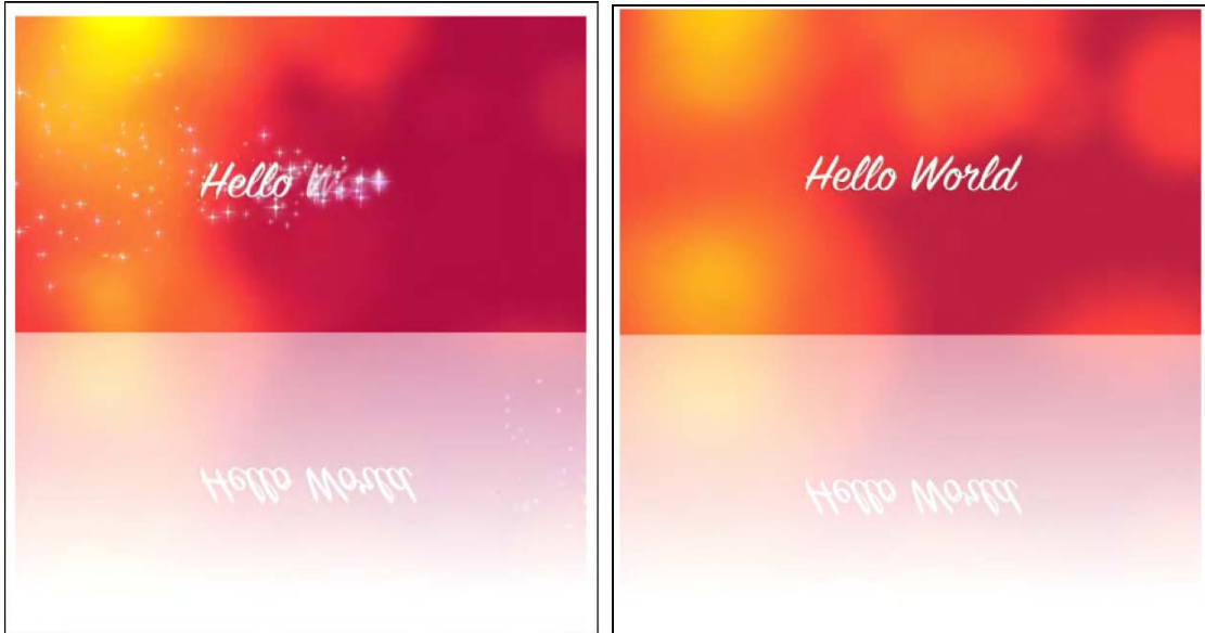
Figure 5–16. Rendering inline SVG with reflection on video in Firefox (left) and Opera (right)
