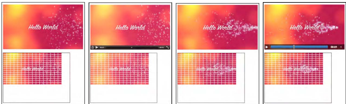
Figure 6–6. Attempted tiling of a video into a canvas using putImageData() in Firefox, Safari, Opera, and Google Chrome (from left to right).
