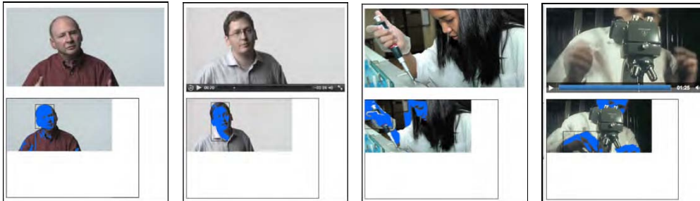
Figure 7–6. Face detection results on a skin color detected video in Firefox, Safari, Opera, and Chrome (left to right)
