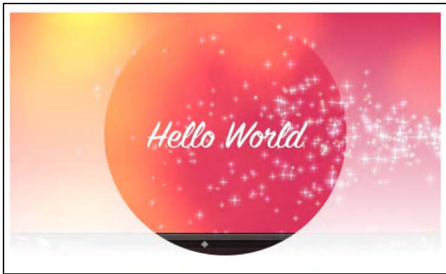
Figure 5–6. An SVG mask and a gradient applied to a video in Safari and Firefox shows the same effect
