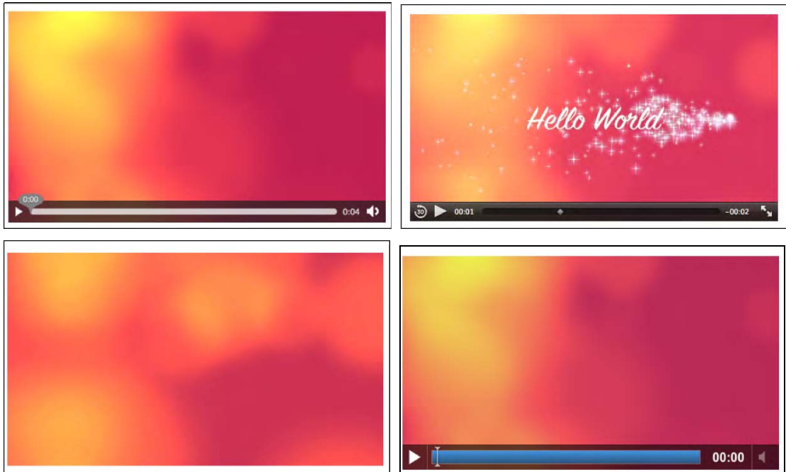
Figure 5–14. Rendering inline SVG with video in Firefox (top left), Safari (top right), Opera (bottom left), and Google Chrome (bottom right).
