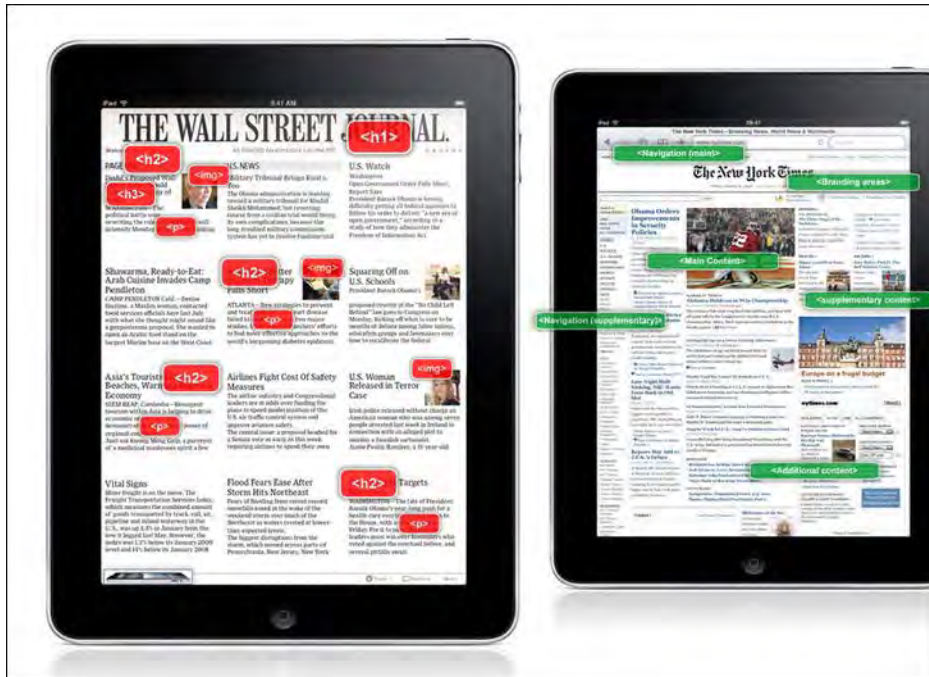
Figure 2–7. HTML W3C compliant markup (left) and its semantic markup implementation (right) on the Wall Street Journal and New York Times web sites
