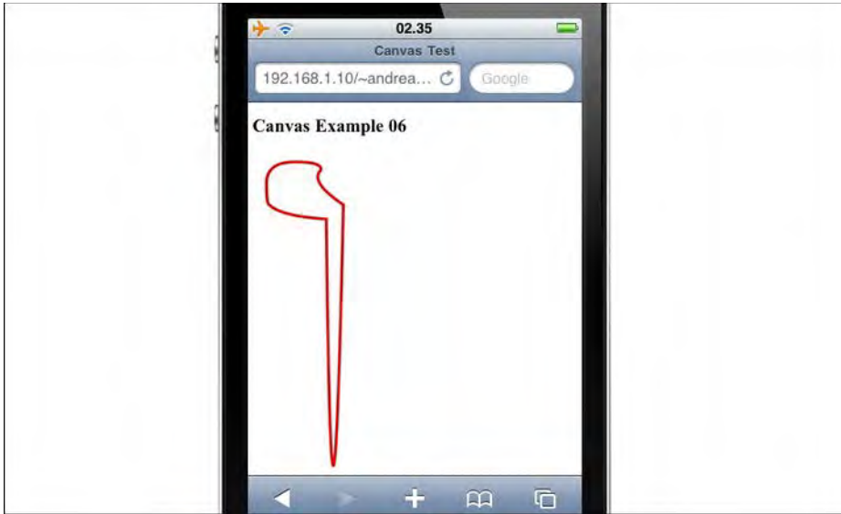
Figure 7–10. The HTML 2D API in action: drawing using quadratic curves
