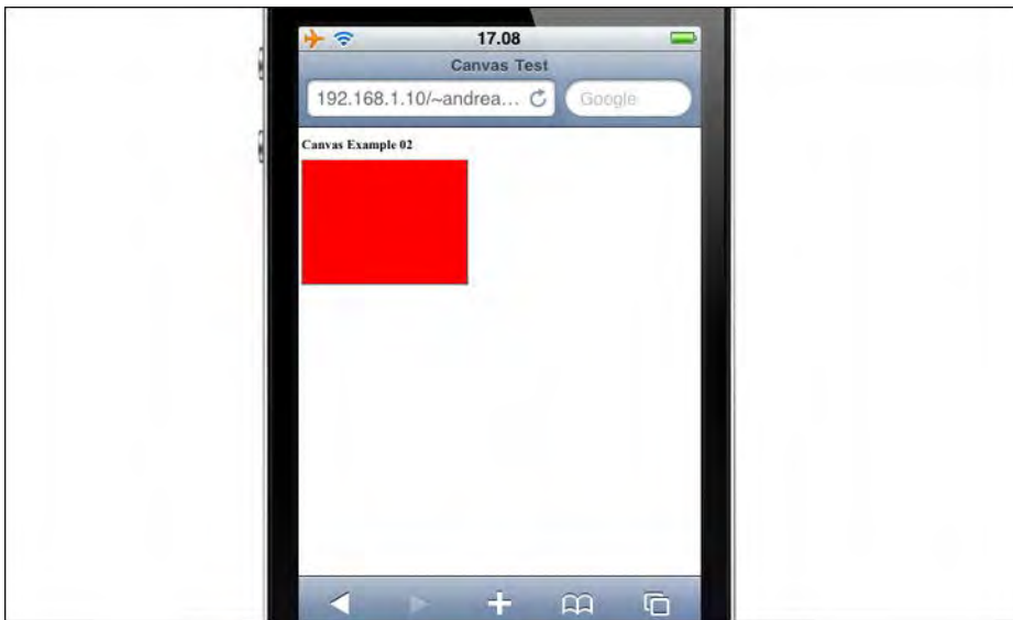
Figure 7–5. The HTML 2D API in action: drawing a basic shape using Canvas and Methods
