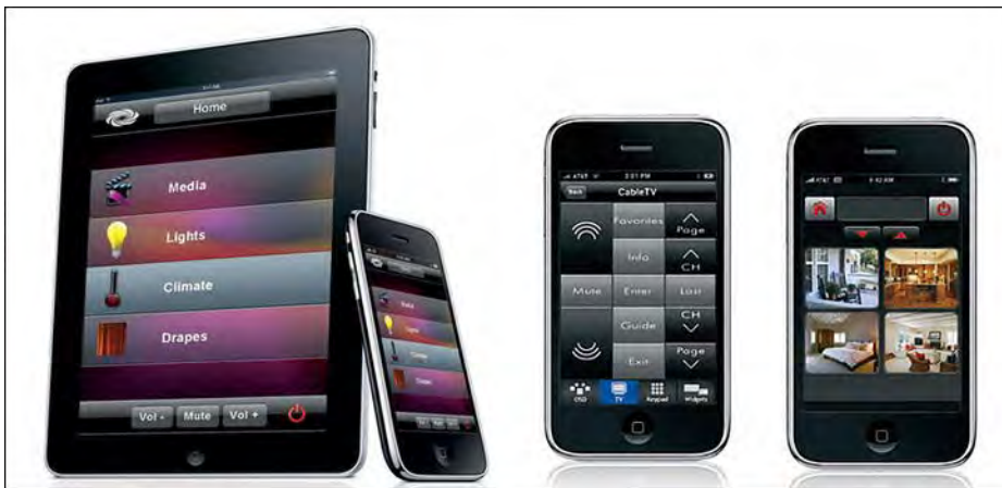
Figure 13–3. Crestron (left) and Savant (right) applications for home automation
