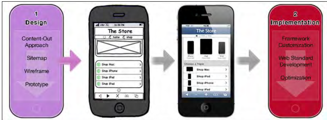
Figure 11-3. The paper test performed between the design and the implementation phases of the flow.
