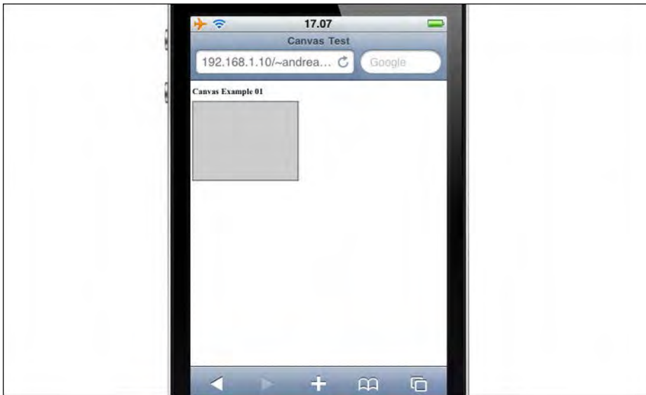
Figure 7–3. The HTML 2D API in action: drawing a basic shape using Canvas and CSS
