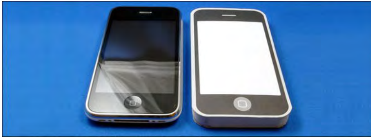
Figure 2–14. A paper prototype tool compared with a real iPhone
