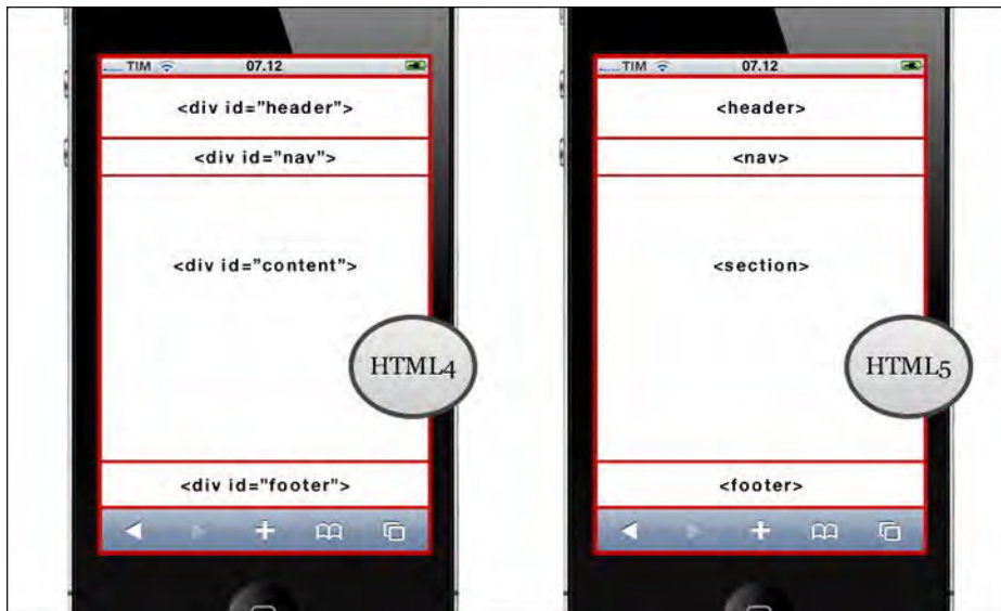
Figure 7-1. HTML4 and HTML5 comparison in two simple iPhone page structures
