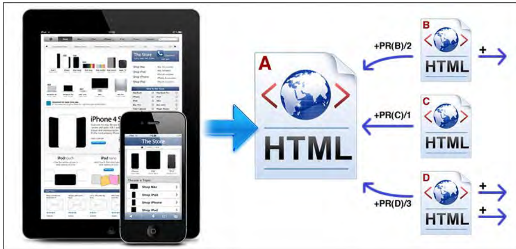
Figure 10–12. The Google Page Rank Algorithm: web page B, C, D add their PageRank value to web page A
