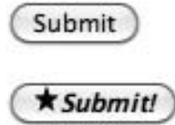
Figure 4-17. Two submit buttons, one created with the input element (top) and the other created with the button element (bottom)
