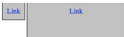
Figure 6-15. Inline-level box and block-level box being treated as an inline-level box for layout purposes
