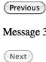
Figure 7-4. The output of a simple Ajax application after two clicks of the next button. The button is disabled when the last of the three messages is displayed.
