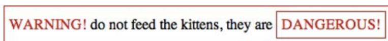
Figure 6-3. Class style rules can be “doubled up” on each other by setting more than one styled class attribute value on an element.
