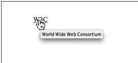
Figure 2-2. The tool tip effect of the title attribute being set on a link
