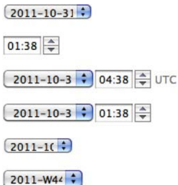
Figure 4-10. All the different date- and time-related inputs as shown in the Opera web browser. From top to bottom: date, time, datetime, datetime-local, month, week.
