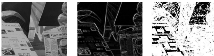
Fig. 5. Left : Venus test image, Center : Edge detection result(Amount of pattern) Right : Binarization image ( Threshold = 10)
