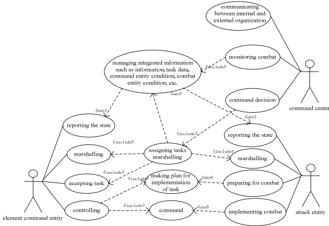
Fig. 3. Use case diagram of Network-Based C2 System
