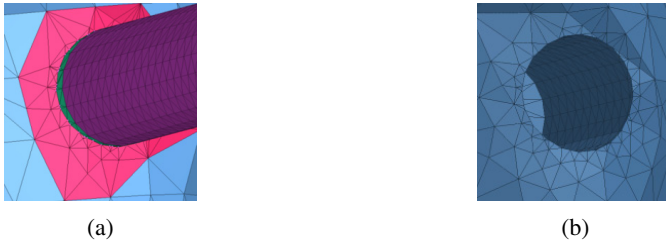
Fig. 6. Inserting implant. (a) Divided regions depending on the intersection curve. (b) Combined regions to insert implant.
