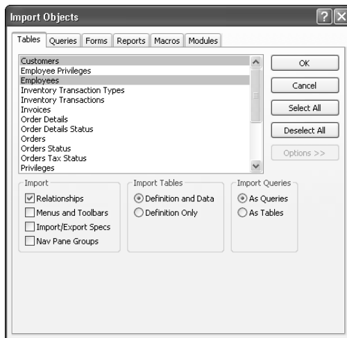
Figure 4-8: The Import Objects dialog box allows you to import database objects from another Access database.
