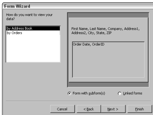
Figure 1-5: The Form Wizard can create a form with a subform for information from a related table or query.
