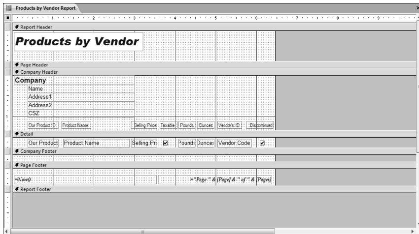
Figure 1-13: Report sections determine what prints at the beginning and end of the report, in each section of the report, and at the top and bottom of the page.
