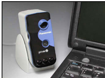
Figure 2. Panasonic BM-ET100US authenticam iris recognition camera
