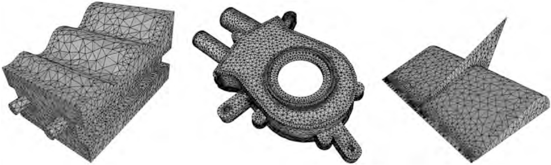
Meshing Piecewise Smooth Complexes, Fig. 1 Example meshes of PSC: (left) a piecewise smooth surface, a non-manifold, a surface with non-trivial topology
