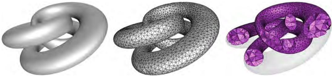
Smooth Surface and Volume Meshing, Fig. 1 A knotted torus, its surface mesh, and its volume mesh
