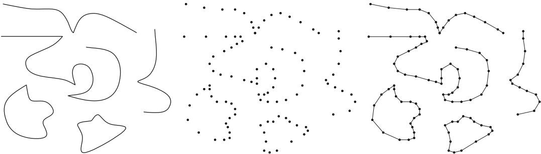
Curve Reconstruction, Fig. 1 A collection of curves \Gamma , a sample S from \Gamma , and the correct reconstruction G(S, \Gamma)
