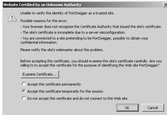
Figure 19-4: Using an intercepting proxy with HTTPS communications generates a warning within the attacker's browser.
