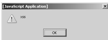
Figure 12-2: A proof-of-concept XSS exploit
