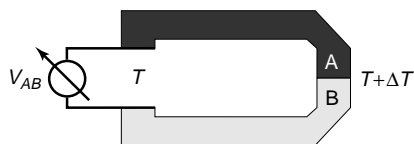
Figure S.4 Schematic of Seebeck effect.
