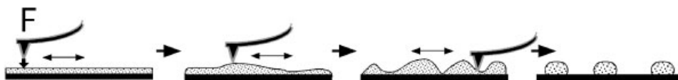
Fig. 5.9 Schematic of the patterning mechanism of rotaxane thin films upon mechanical perturbation of an AFM tip.
