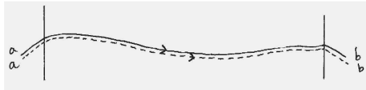
Fig. 6. The conductance is proportional to the classical probability to transmit channel a to channel b (summed over channels). The object which represents this probability is the sum of contributions of paired trajectories as introduced in Fig. 4. We call it a “ Diffuson ”
