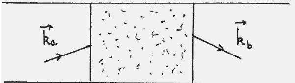
Fig. 5. In the Landauer formalism, the conductance is related to the transmission coefficient between different incoming and outgoing channels
