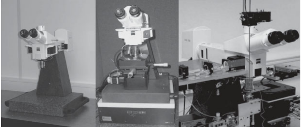
Fig. 8.1 Base construction of the optical microscope and some add-on SPM systems.
