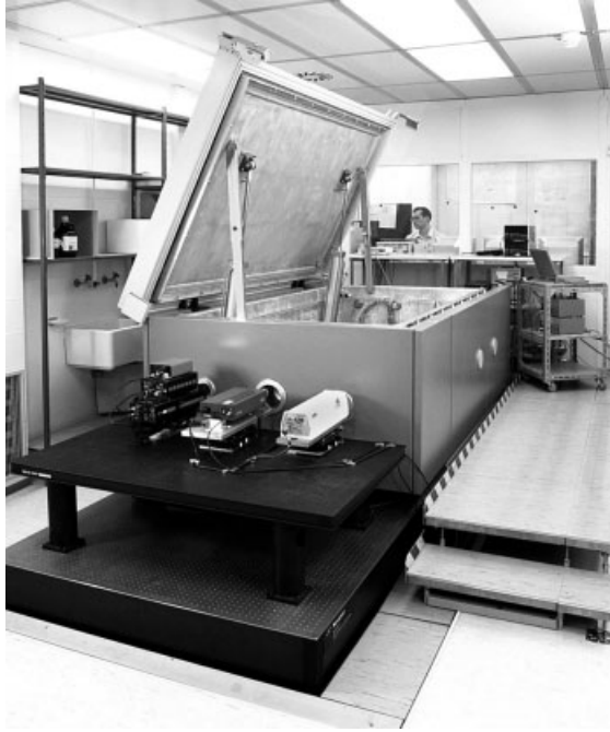
Fig. 26.1 Comparator for the calibration of complete LIs with measuring chamber.
