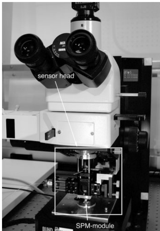
Fig. 1.5 View of the combined SFM and interference microscope composed of sensor head and commercial basic instrument.
