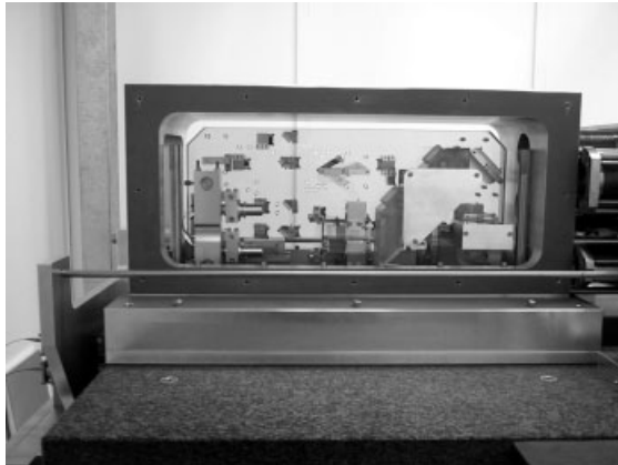
Fig. 30.3 Photo of the interferometer beamsplitter in the vacuum chamber.
