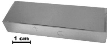
Fig. 18.11 Quartz glass with 10 nm platinum coating (60 mm x 20 mm x 10 mm).
