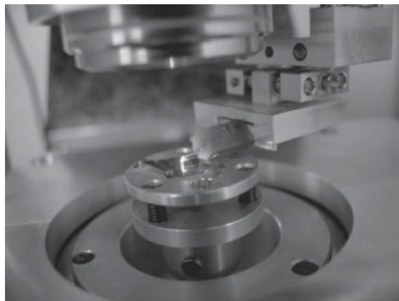
Fig. 8.6 View of the SPM head: tuning fork holder with the tuning fork and its glued diamond tip.
