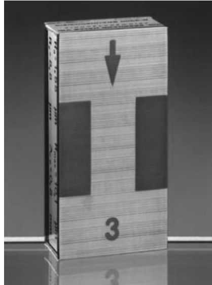
Fig. 6.11 The photo of the measured PTB micro roughness standard. Size: 40 mm (L) \times 20 mm (W) \times 10 mm (H).
