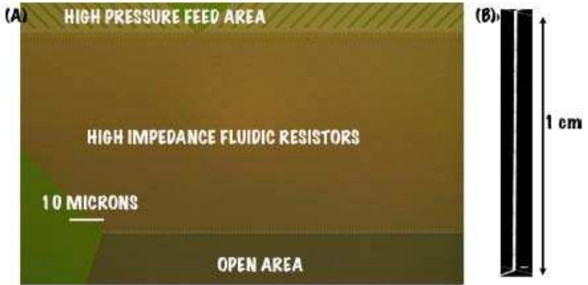
Figure 3.3 (A) Corner of an etched device consisting of a wall of current injectors. (B) Laminar jet of fluorescent 1.0 micron balls propagating through an open area, with flow determined by the boundary conditions.
