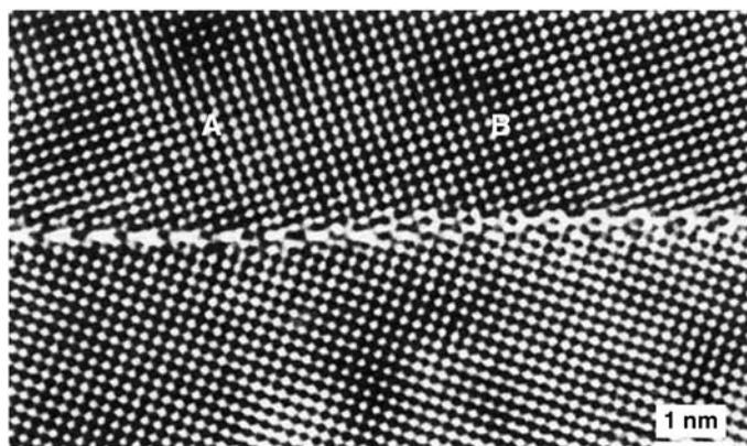
Figure 1.14 Atomic-resolution electron micrograph showing a \Sigma = 5 , (310) symmetric tilt grain boundary in NiO recorded close to optimum defocus (black atomic columns). Note the change in geometry of structural units as boundary translates from region A to region B. Reproduced from Ref. 55.
