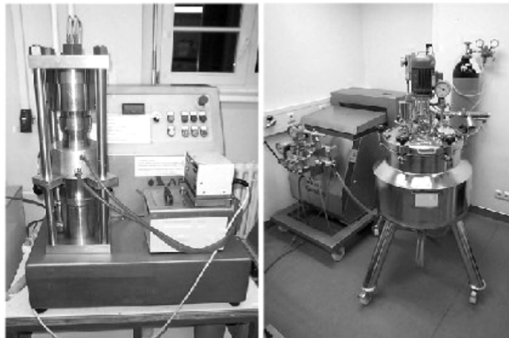
Figure 3-2. APV LAB 40 for batch sizes up to 40 mL (left) and Gaulin 5.5 in series with feeding container (150 kg / hour) (right).
