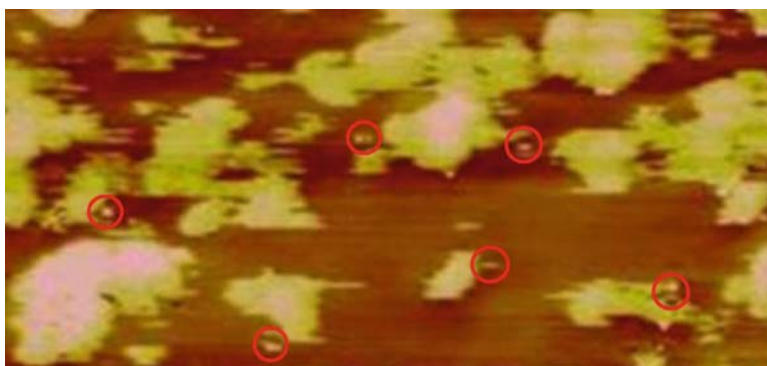
Fig. 14.10 Test of the EFM on indium tin oxide clusters deposited on a silicon surface at a bias voltage of 3 V. The smallest features visible in this image ( red circles ) are individual clusters with feature sizes of 30 down to 10 nm. This proves the very high resolution that can be obtained with our EFM setup
