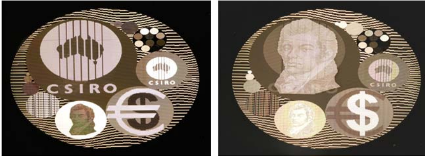
Fig. 7.35. Photographs of the images generated by a nickel shim containing a two-channel micromirror OVD with a grayscale portrait image in one channel. The diameter of the OVD is 36 mm
