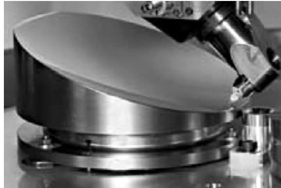
FIGURE 11.16 An off-axis parabolic mirror machined on the LODTM. [ http://www-eng.llnl.gov/lohtm/success_pg2.html (accessed December 2003).]
