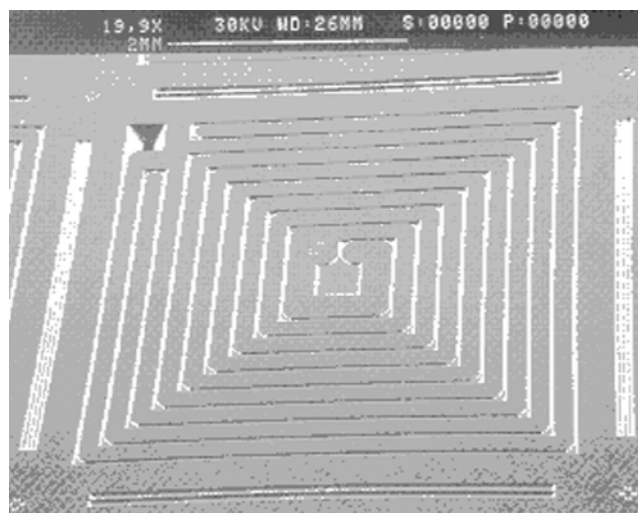
FIGURE 12.10 Scanning electron micrograph of a microflow restrictor showing an array of diamond coated V-type channels. (Courtesy of CSEM, Switzerland.)
