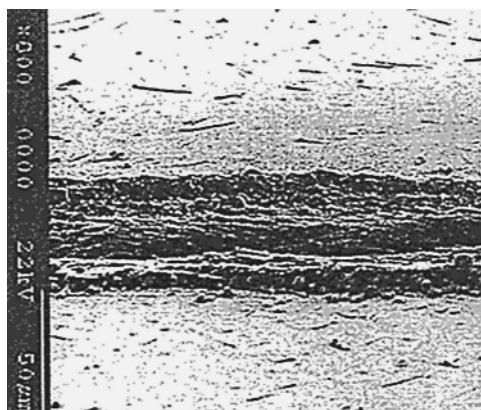
FIGURE 8.12 Trench machined in steel created using a nanosecond-pulsed Nd:YAG laser in an air-rich gas atmosphere. (Jackson, M.J., G.M. Robinson, B. Mills, and W. O'Neill, Proc. Inst. Mech. Eng. Lond. B J. Eng. Manuf. , 217, 553–562, 2003.)
