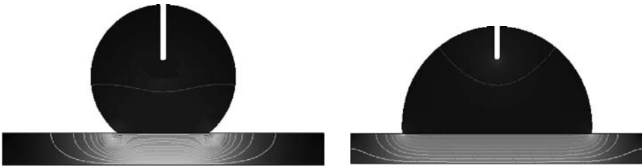
Figure 4.21 The amount of stored electrical energy decreases with the contact angle. Left: large contact angle; right: smaller contact angle. The contour lines correspond to the electric potential (calculation performed with the COMSOL numerical software).
