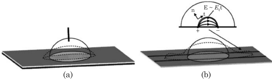
Figure 4.13 Two different configurations for electrowetting experiments: (a) Static change in the macroscopic contact angle obtained using dielectric film coated planar electrodes; (b) electrowetting effect produced using parallel line electrode configuration. The inset shows a schematic representation of the cross section of the bulk drop and electrowetting film showing that the electric field lines are predominantly tangential to the interface. From [21]. © 2006 APS; reprinted with permission.
