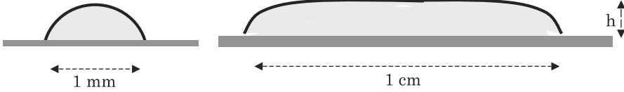
Figure 3.1 Comparison of the shape between micro-drops and macro-drops (not to scale): micro-drops have the shape of spherical caps whereas larger drops are flattened by the action of gravity and their height is related to the capillary length.
