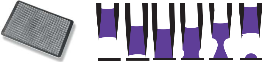
Figure 2.1 (a) View of a microplate for Biotechnology applications, from [1]. © 2004 JALA. Reprinted with permission. (b) Capillarity is a determining force when spotting a droplet on a microplate, from [2].
