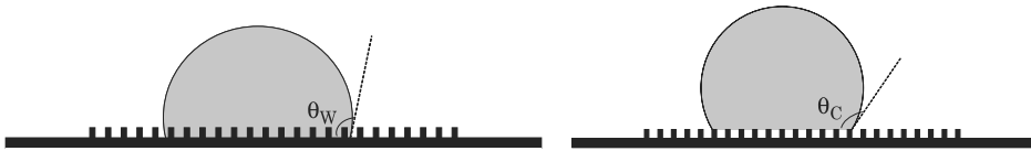
Figure 3.49 Left: droplet penetrating between the pillars, right: droplet sitting on top of the pillars (fakir effect). \theta_W is the Wenzel contact angle and \theta_C is the Cassie contact angle.
