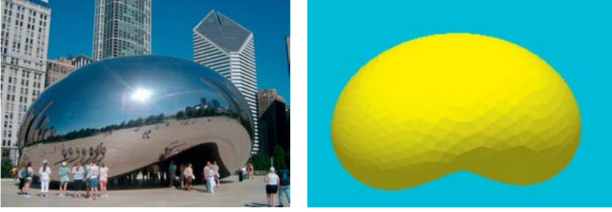
Figure 2.77 Left: striking example of minimal surfaces in Architecture: the “Cloud Gate” sculpture by Anish Kapoor in the Millennium Park of Chicago. Right: calculation of a similar surface with the Surface Evolver numerical software (right).
