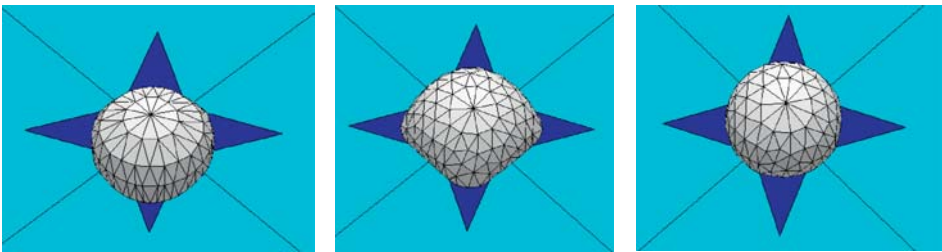
Figure 5.55 Surface Evolver simulation of a droplet on a star-shaped electrode. Left: the droplet is initially positioned arbitrarily on the plane; middle: when the star-shaped electrode is actuated, the droplet moves in such a way that it maximizes its contact surface on the actuated electrode; right: after the actuation is turned off, the droplet regains its spherical shape and is positioned at the center of the star-shaped electrode.
