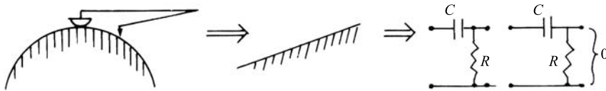
Figure 4.101 Use of skid system and electrical filter to remove curves.
