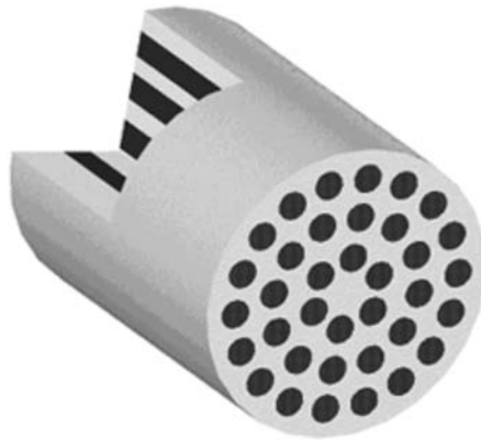
FIGURE 21.7 Typical bicomponent islands-in-the-sea fiber.
