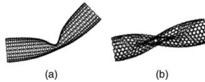
FIGURE 23.9 (a) Buckling of SWCNT under bending load. (b) Buckling of SWCNT under torsional load.
