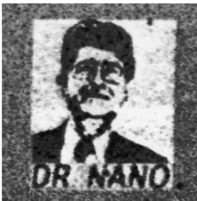
FIGURE 3.D1 This nanograph of Dr. M. Roco was recorded at Oak Ridge National Laboratory using piezoresponse-force microscopy, one of the members of the family of techniques known as scanning probe microscopy, which can image and manipulate materials on the nanoscale. Each picture element is approximately 50 nm in diameter; the distance from chin to eyebrow is approximately 2.5 \mu\text{m} .
