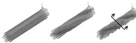
FIGURE 23.31 Snapshots of twisting of the SWCNT bundle. The twisting angles are 30, 60, 90, 120, 150, and 180 degrees, respectively.
