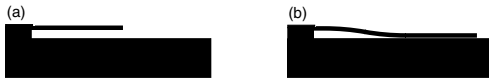
Fig. 14.5. a Micrometer sized cantilever beam. b If the beam is too long or too thin the minimum free energy state corresponds to the beam partly bound to the substrate. Surface roughness lowers the binding energy (per unit area) and hence stabilizes the non-bonded state in a
