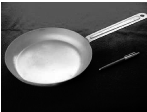
Fig. 14.1. A stainless steel pan coated by a quasicrystal material. The coating was made using electron beam vapor deposition in vacuum
