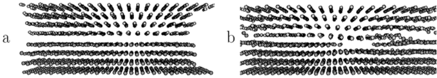
Fig. 10.4. a Low-load configuration of chemically-passivated solids with terraces. Both solids are fcc Lennard Jonesium with [111] surfaces. The surfaces are mis-oriented by 90^\circ . Static and kinetic friction are too small to be defined, because thermal fluctuations at ambient conditions are strong enough to depin the contact. b Snapshot of a configuration that results from configuration a as a consequence of high normal pressure. Despite the onset of plastic deformation, the static friction coefficient for this contact remains smaller than 0.01. From Ref. [26]
