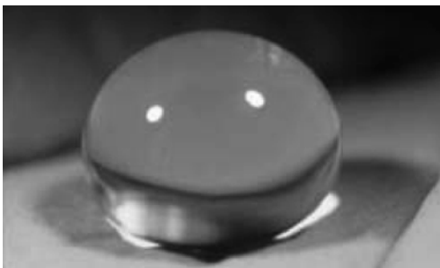
Fig. 14.6. A water droplet on a superhydrophobic surface: The droplet touches the leaf only in a few points and forms a ball. It completely rolls off at the slightest declination. From [10]
