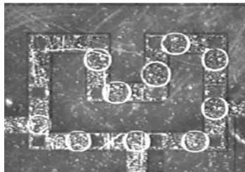
Fig. 2. Droplet transport in a two-dimensional array. (detailed video available at http://www.ee.duke.edu/Research/microfluidics )
