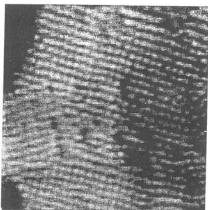
Fig. 6. 28\text{ nm} \times 28\text{ nm} STM image of a monolayer of \alpha\text{-SiW}_{12}\text{O}_{40}^{4-} on an Ag(111) surface in 0.1\text{ M HClO}_4 . I_{\text{tip}} = 2.7\text{ nA} , E_{\text{tip}} = 100\text{ mV} .
