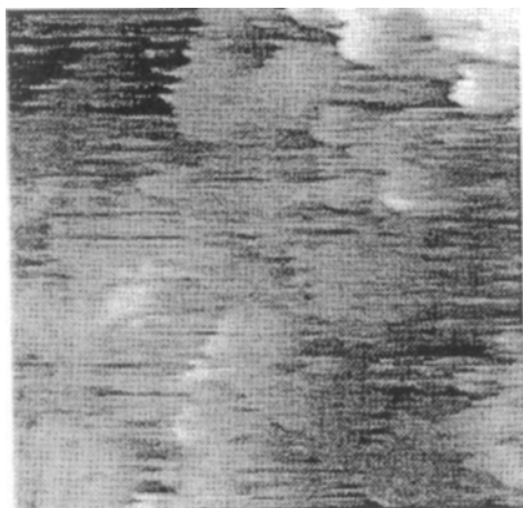
Fig.2. Example of an irreproducible STM picture of fine-grain titanium covered with 20nm \text{TiO}_2 , xy range: 75 \mu\text{m} , -3 V bias, -1 nA setpoint, z_{\text{max}} = 643 nm, scan rate 100 \mu\text{m/s} , W tip, normal air. Horizontal white or black lines between homogeneous areas indicate feedback irregularities.
