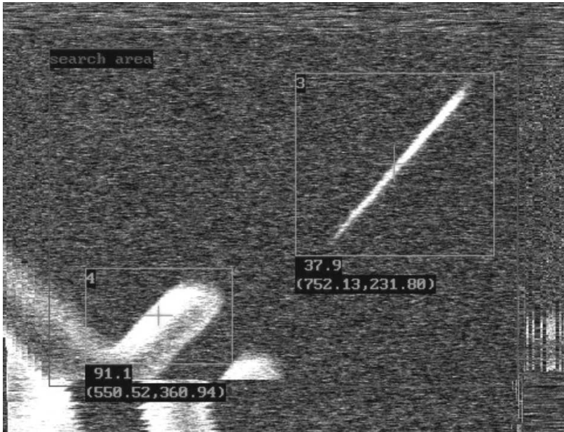
Figure 4.6. Tracking of a gripper tip and a CNT using cross-correlation and an adaptive ROI. The length of the CNT is 6 \mu\text{m}
