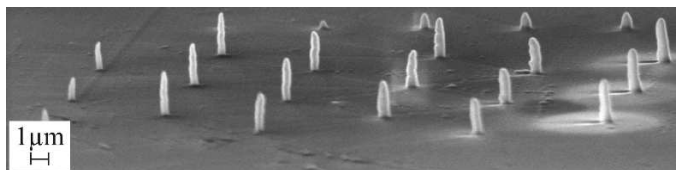
Figure 10.7. Example of EBiD deposits on a silicon wafer from a tungsten-hexacarbonyl precursor. These “pins” have been deposited by pointing the SEM’s electron beam on one spot for several minutes.
