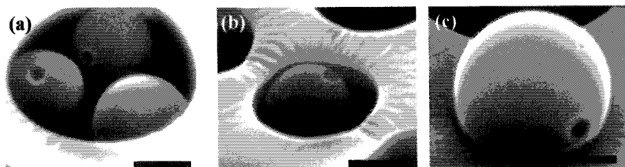
Fig. 3. Scanning electron micrographs of the combination of PS particles and titania honeycomb films. (a) 1.5 \mu\text{m} PS particles in a 3.3 \mu\text{m} honeycomb pore. (b) A single 1.5 \mu\text{m} PS particle in a 2.7 \mu\text{m} honeycomb pore. (c) A 3.2 \mu\text{m} PS particles capped over a 2.7 \mu\text{m} honeycomb pore. Each black bar indicates 1.0 \mu\text{m} .
