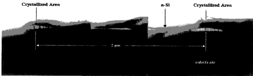
Fig. 6. The cross-section TEM photographs of two adjacent crystallization regions in ultra-thin a-Si single layer after LIC with energy density of 39 \text{ mJ/cm}^2 in front of 2D grating. The substrate is \text{SiN}_x/\text{Si} .
