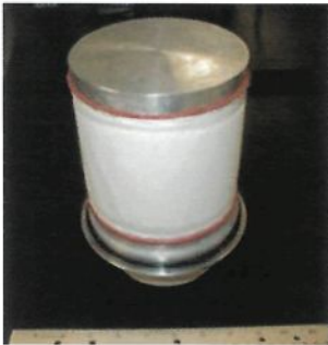
Filter membrane on the surface of the perforated tube
