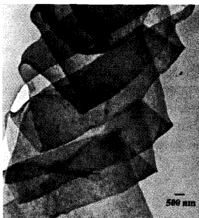
Fig. 28. TEM micrograph of a ribbon shaped nanofiber. Reprinted from [75], P. H. Fong et al. , Polymer 43, 775 (2002) © 2002, Elsevier Science.
