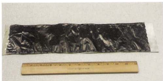
Fig. 11. World's largest magnetically aligned buckypaper (17.3 Tesla magnetic field).
