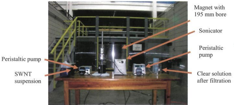
Fig. 10. Modified experimental setup for producing large magnetically aligned nanotube buckypapers.
