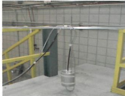
Final filter assembly with suspension supply and outlet tubes
