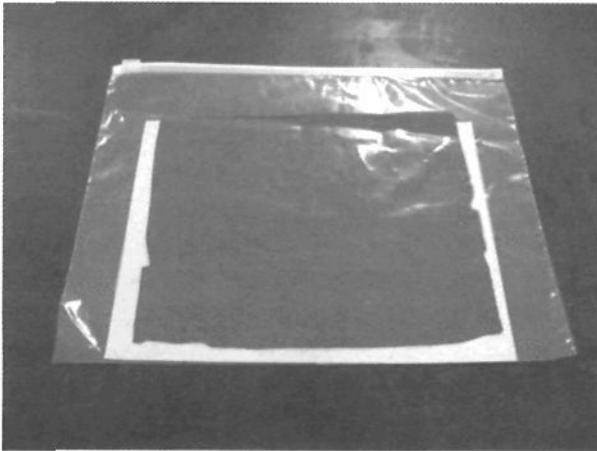
Fig. 7. 9 in \times 9 in randomly oriented SWNT buckypaper.
