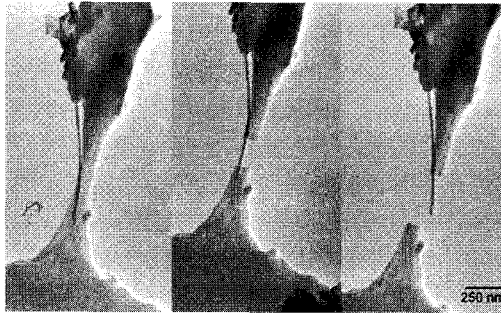
Fig. 14. A weak interaction between the epoxy matrix and the nanotube leads to easy pull-out [65].
