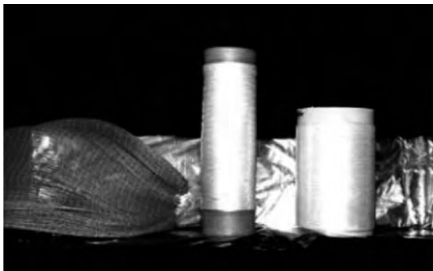
Fig. 6.6. Products made from NPA6 materials (left to right: threads and fibers; films are shown at the back).
