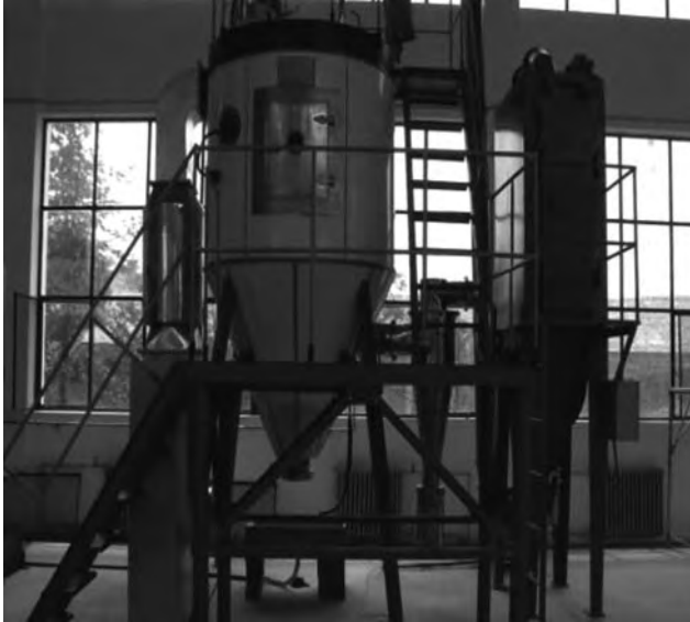
Fig. 6.18. The partial device for preparing MMT powder in industry.
