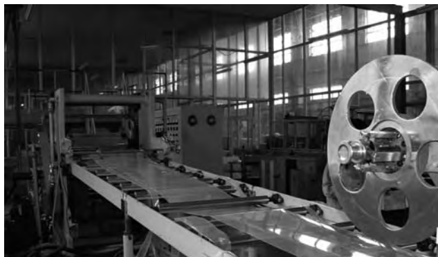
Fig. 6.21. Processing line for plate materials of polypropylene-silica nanocomposites.
