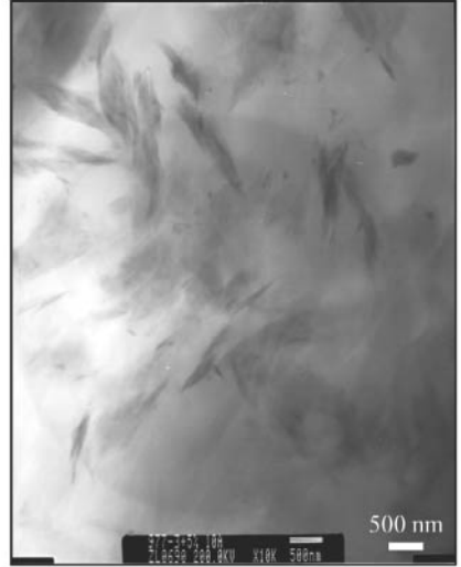
Figure 7.93 Low-magnification TEM micrographs of 977-3/Cloisite 10A (5%) showing uniform dispersion of nanoclay Cloisite 10A in 977-3 epoxy resin, where scale bar is 500 nm.
