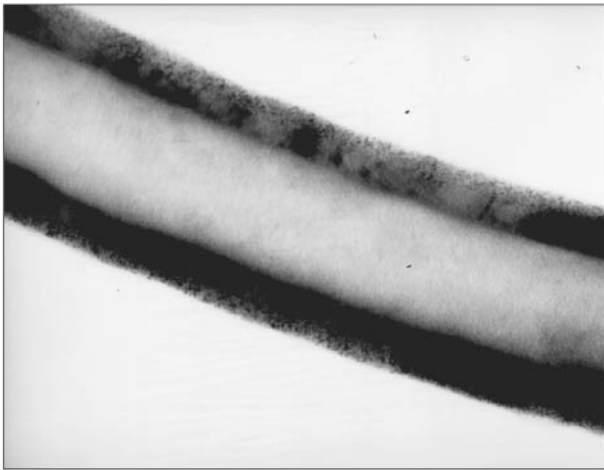
Figure 2.15 TEM micrograph showing carbon nanofibers have a hollow core and two distinct regions, catalytic and deposited. (Courtesy of ASI.)
