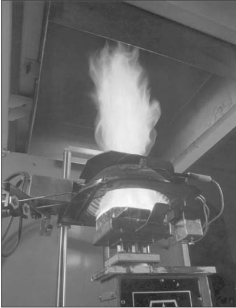
Figure 5.9 Close-up showing test specimen igniting during Cone Calorimeter testing.
