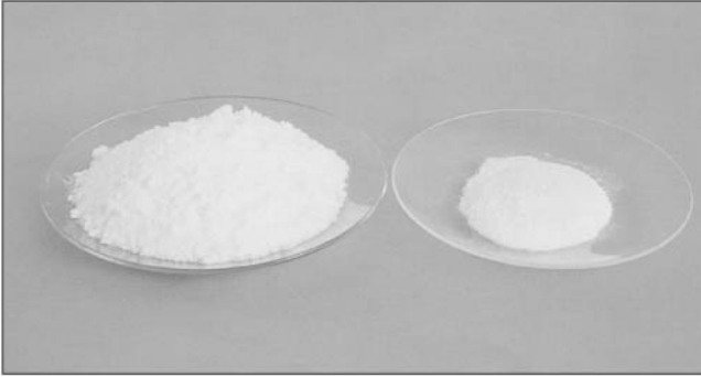
Figure 2.41 Comparison of 10 g of commercial Aluminum Oxide C (compacted apparent density about 80 g/L) (left) and 10 g of Aluminum Oxide C compacted by the wet process (compacted apparent density about 550 g/L) (right). (Courtesy of Degussa.)
