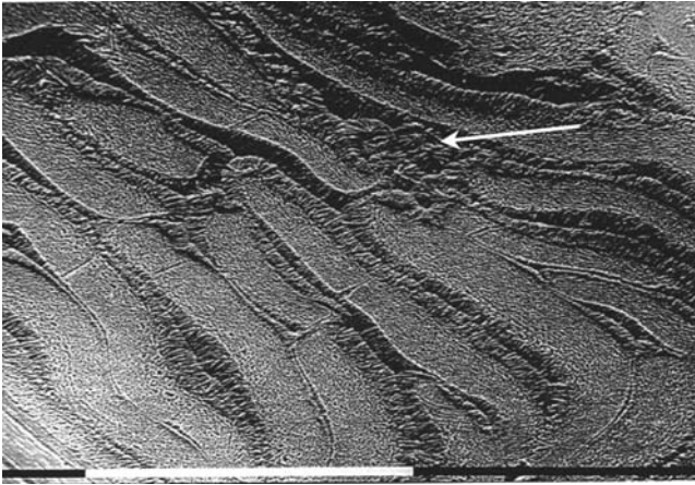
Figure 12 Etched SEM micrograph of compacted polypropylene fibrillated tapes showing crystallization nucleating between the tapes (white arrow) as well as at the tape surfaces. (From J. Teckoe, R.H. Olley, D.C. Bassett, P.J. Hine and I.M. Ward, J. Mater. Sci. , 34, 2065–2073, 1999. With permission.)
