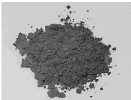
Figure 2.6 Powder of PANI prepared by mechanochemical method for 1 h [41]
