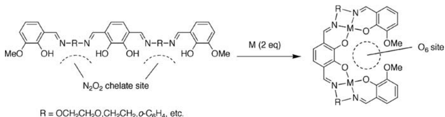
Scheme 10.6. Regulation of ion recognition by metalation of bis( N_2O_2 ) chelate
