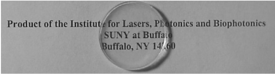
Figure 6.3. Photograph of an up-converting transparent glass laid over the writing to show its clarity.
