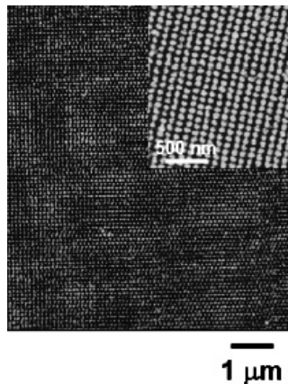
Figure 11.21. AFM topographic images of an etched MHA/Au/Ti/SiO x /Si dot nanoarray. From Zhang et al. (2003), reproduced with permission.
