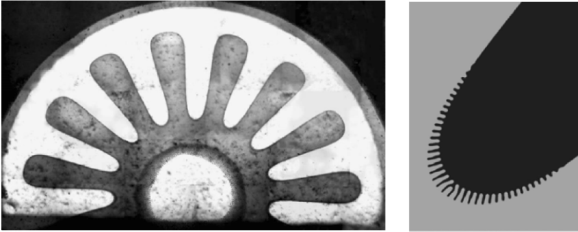
Figure 10. Multipole axially magnetized microrotor ( \phi 8 mm) as imaged by an uniaxial MOIF. Enlarged fragment (right) shows the DW sinusoidal instability developing with the decrease of the field gradient.
