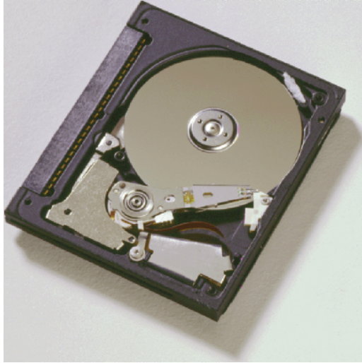
Figure 3. IBM microdrive, 2000 \times 10^6 kBit/in 2
