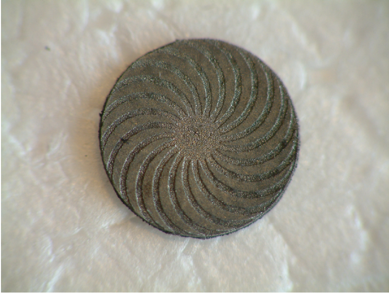
Figure 2. Bulk micro-machined NdFeb rotor with etched planar turbine
