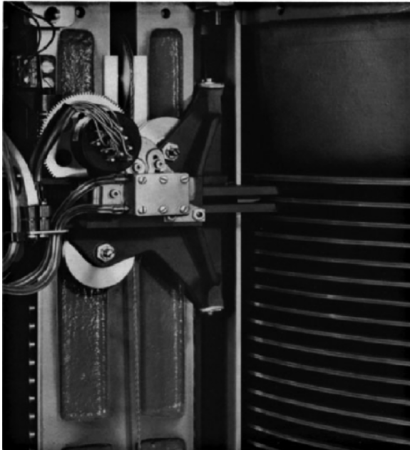
Figure 2. IBM Type 350 hard disc, 1956 2 kbit/in 2
