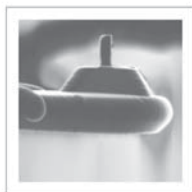
(C) Repeating the diametrically opposed cuttings at the front areas of the pyramidal tip, after a 90^\circ turn of the cantilever.
