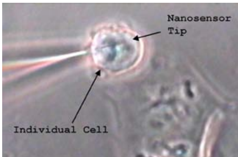
Fig. 7. Monitoring of single human mammary carcinoma cell using fiberoptic nanosensor.
