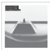
(E) Final milling step in order to remove deposited material.
