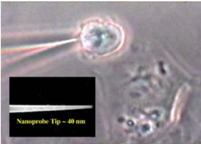
Fig. 7. Fiberoptic nanosensor for single-cell analysis. (Adapted from ref. 10. )
