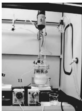
FIGURE 5.3 Experimental setup for semicontinuous emulsion polymerization.
