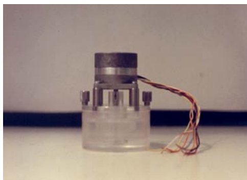
Figure 4.46. Prototype of industrial reactor, consisting of a rotating pilot reactor at laboratory level but displaying deposition industrially feasible (Reprinted with the permission from Nicolini and Pechkova, Nanostructured biofilms and biocrystals, Journal of Nanoscience and Nanotechnology 6, pp. 2209–2236 © 2006a, American Scientific Publishers, http://www.aspbs.com ).
