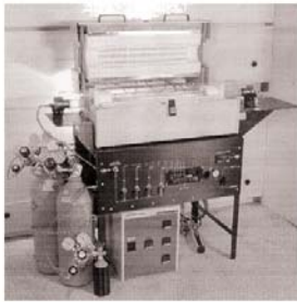
A. CVD system SW/MWNTs deposition
