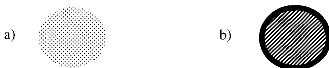
Fig. 2 Schematic representation of a) nanospheres, drug homogeneously distributed within the matrix, and b) nanocapsules, drug-core surrounded by shell.
