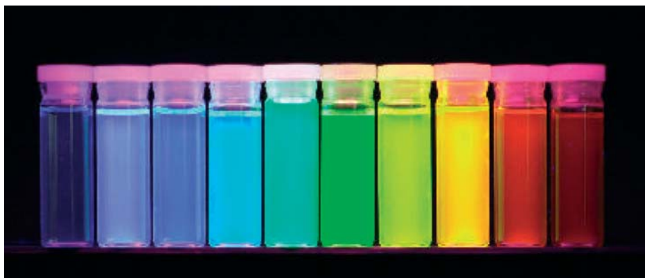
Figure 22.1 Ten distinguishable emission colors of ZnS-capped CdSe quantum dots excited with a near-UV lamp. From left to right (blue to red), the emission maxima are located at 443, 473, 481, 500, 518, 543, 565, 587, 610, and 655 nm.
