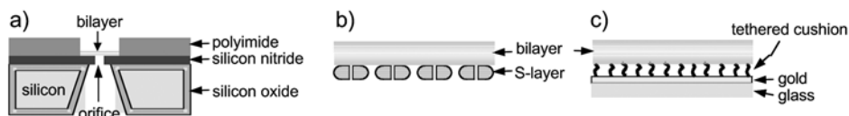
Figure 7.7 Different classes of robust bilayer. (a) Bilayer across a small aperture formed in silicon nitride [83]. (b) Bilayer on a porous support comprising a bacterial S-layer [84]. (c) Tethered supported bilayer on a smooth gold surface [86].
