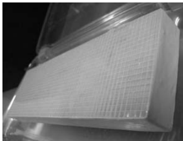
Figure 2. Inorganic scintillator crystals arrays. The size of the crystal is 2.2 \times 2.2 \times 15 \text{ mm}^3 and that of the arrays is 140.8 \times 44 \text{ mm}^2 .
