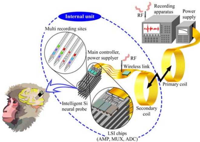
Figure 1. Configuration of intelligent Si neural probe system.
