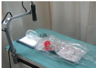
Figure 1. Surgical simulator for endovascular neurosurgery fabricated by a photoelastic modality, allowing for the evaluation of stresses on the arterial structure applied during surgical procedures and blood streaming.
