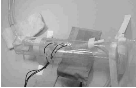
Figure 5. A photograph of the pressure sensors for Pulse diagnosis and model circulation of a radial artery
