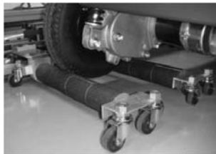
Figure 3. Lifting of the wheel using two bars.
