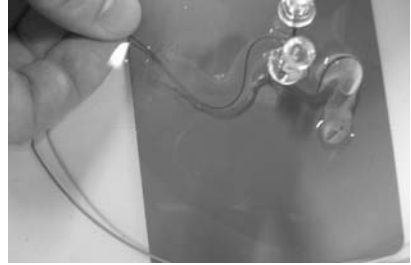
Figure 6. Guidewire in tubular PVA-H model with a realistic geometry.
