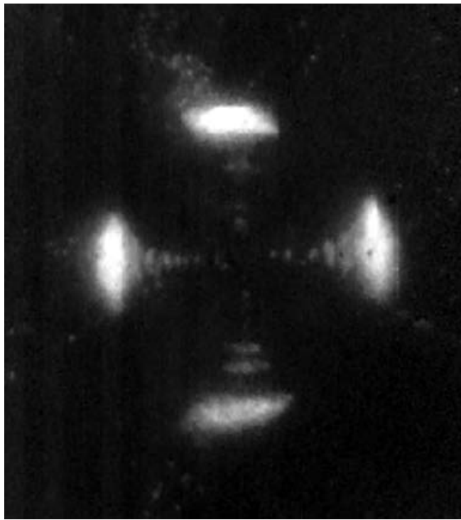
Figure 4.7 The collection patterns of 512-nm-diameter latex beads near the crossover frequency, observed using evanescent illumination. The particles experience positive collection at 1.5 MHz, but fluid flow pushes them out from the array. Particles form bands of pearl chains between the electrodes, which increases the attraction force. The electrode array is similar in configuration and dimension to that seen in Figure 4.1.
